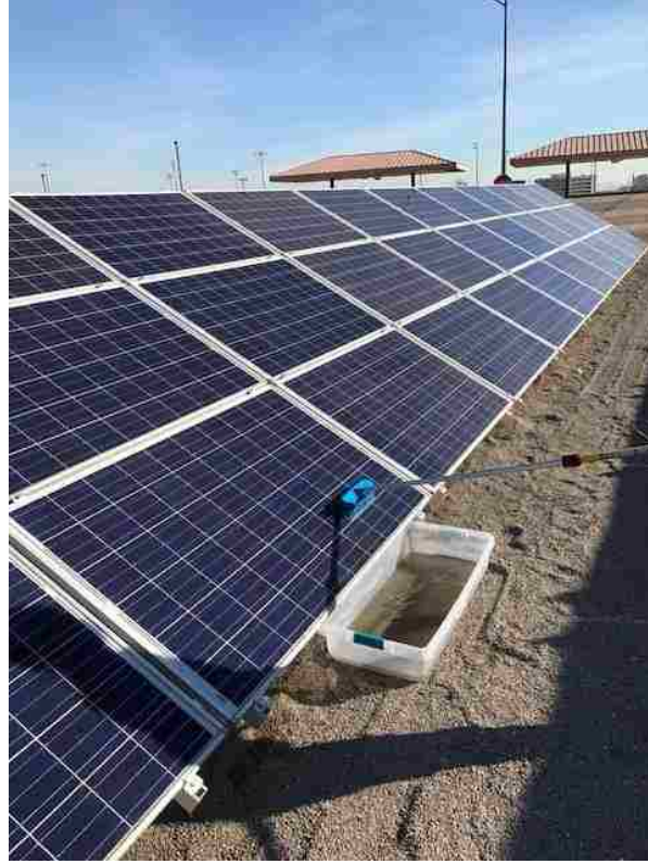
Figure 8. Panel cleaning process using a soft brush and long containers to collect the wash water for analysis
