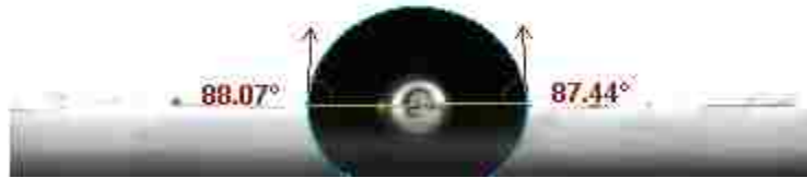
Figure 10. Left and right contact angle located on the surface of the tempered glass sample
