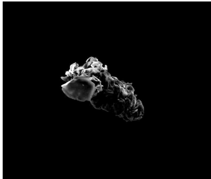
Figure 31. Particle on glass sample from solar panels washed with distilled water
