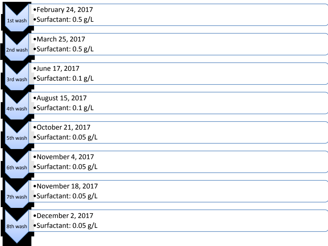
Figure 7. Cleaning schedule and the concentration of the anionic surfactant (Sodium Dodecyl Sulfate) utilized to wash solar panels
